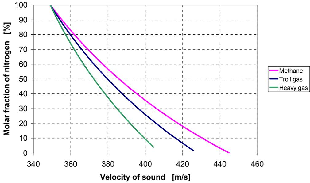
Figure 5 Calculated data for molar fraction of nitrogen as a function of velocity of sound for a mixture of nitrogen and each of three natural gases. Pressure: 1 bara, temperature 20 °C.
