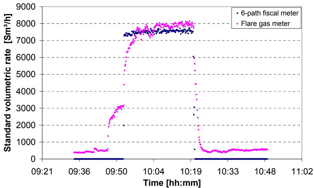
Figure 4 Measured flow rates by the 6-path ultrasonic fiscal flow meter and the ultrasonic flare gas meter during the flow test. Background flaring is not accounted for, and thus the flare gas meter is expected to measure a higher flow rate than the fiscal meter.
