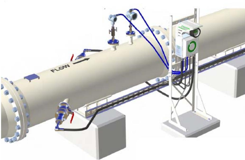
*Figure 2 Typical set-up of an ultrasonic flare gas metering station.*
