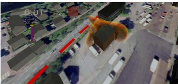
Figure 11. Visualisation of CFD simulation of gas dispersion
