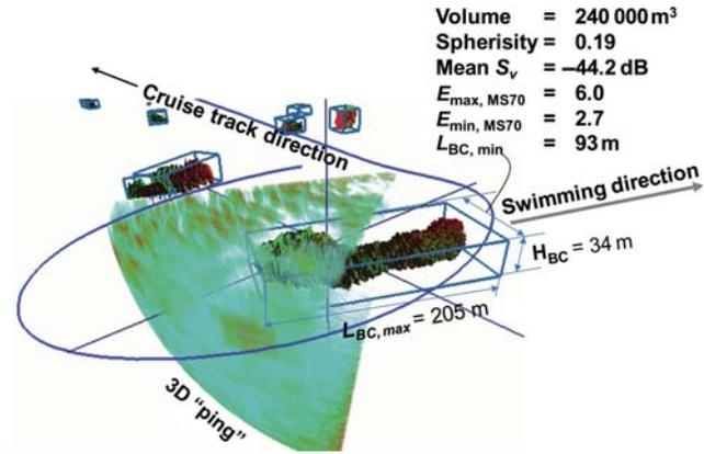
**Figure 4.** A three-dimensional visualization of schools, the cruise track (blue curve), and one MS70 ping partly covering a single school. The schools are detected with several pings. The school is moving in direction from green to red colour (arrow). The bounding boxes are the outer extent of the three-dimensional schools. The quantitative measures are only for the marked school.
