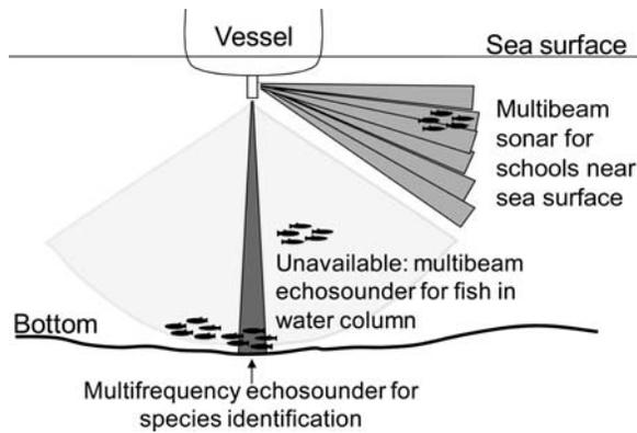
**Figure 1.** Measurements of key ecosystem components with the MS70 sonar and the EK60 echosounders. The gap between the two measurement systems could be filled by a Simrad ME70 multibeam echosounder.
